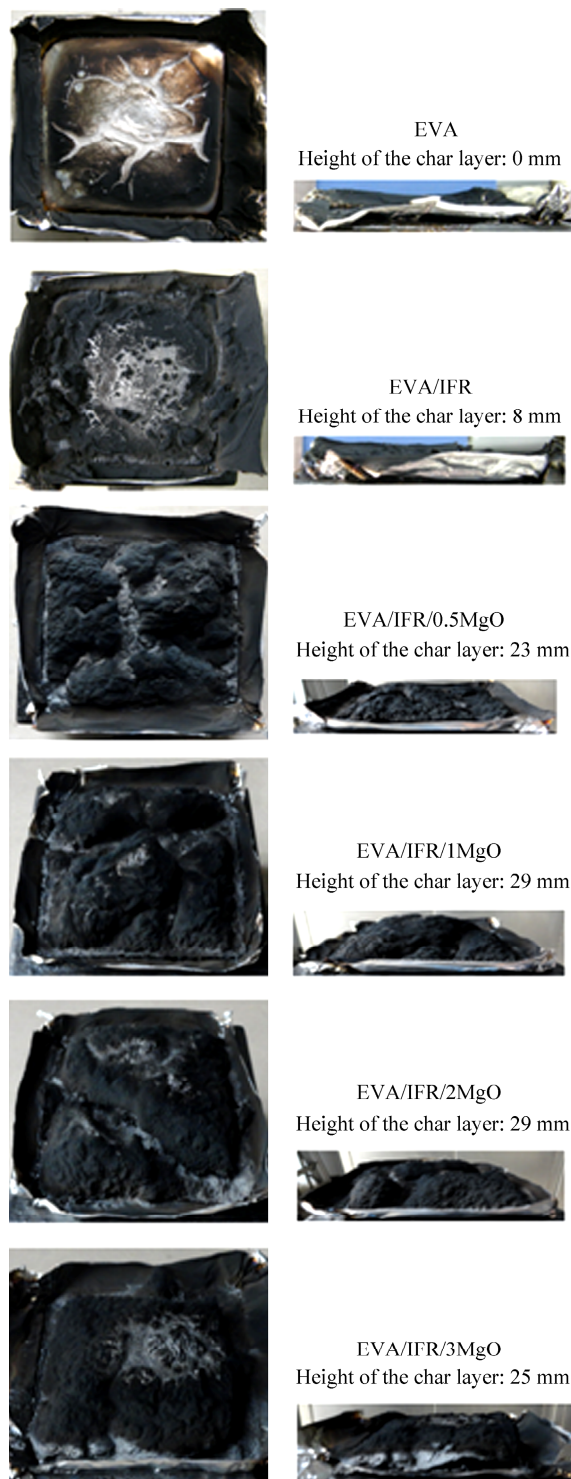
Fig. 2 Optical images of residues after the cone calorimetric test for the flame retardant EVA with IFR and MgO
